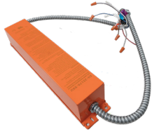
Emergency Driver Item Code: EMD Part #: EHA-EEBB-20W-PANEL 100-277VAC, 50/60Hz, PF>0.9, 300-1,000mA 20V-48V(CLASS 2) 6-20W
